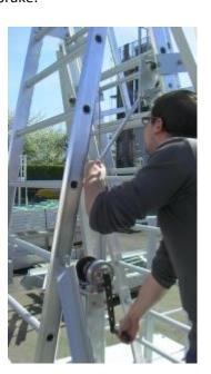
2) Pull the brake handle to maintain the brake in its open position:
