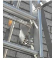
A piece of black plastic round bar is fixed on the cable indicating the end of travel during lifting of the platform. As soon as this piece touches the winch the user MUST stop winding:
